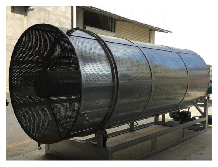
The internal support frame increases the structural strength of the machine and reduces the vibration during use.
