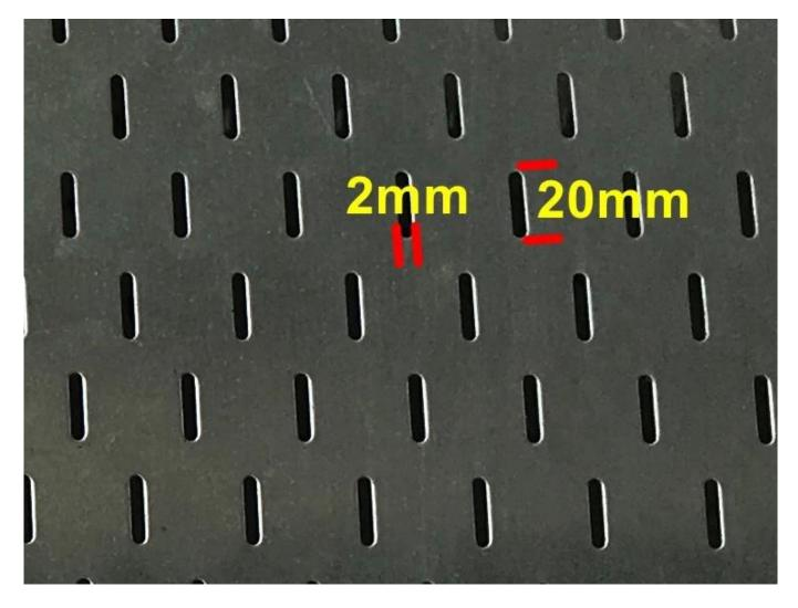
The optimum mesh size obtained by many experiments, the broken tea and tea dusts were screened out during oolong tea shaking process.
