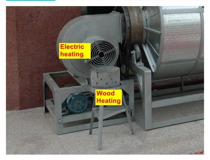
This machine can be heated by electricity or charcoal, If charcoal is used for heating, tea can absorb the taste of charcoal. If charcoal with fragrance is selected, the flavor of tea will be very unique.
