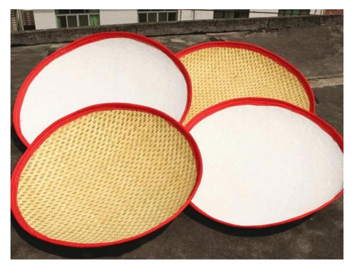
DL-6CRH-120Z made of all bamboo, compared with the cloth covered type, the hole is larger, which is suitable for tea with less powder, and also suitable for the early processing of tea ( withering, fixation, rolling, and fermentation).
