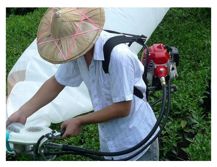
Custom widened and thickened shoulder strap. The width of the strap is widened by 30% and the thickness is increased by 20%. The back board is natural against the waist and conforms to ergonomics, the shoulder and waist will not ache during use.
