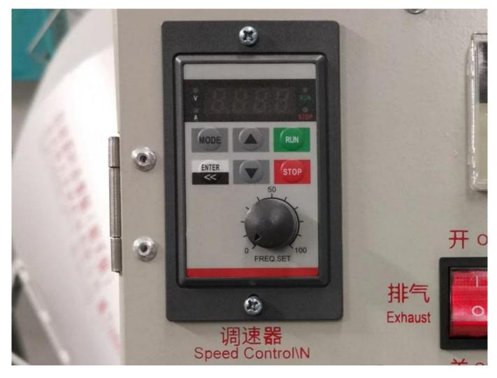
When tea fixation, the speed of the machine can be adjusted, according to the tea of different producing areas, different speed can be adjusted.
