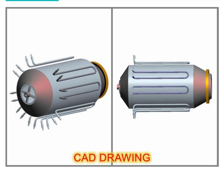
Dense electric heating pipe surrounds the whole fixation drum to ensure the uniform heat of cylinder board, tea fixing more evenly.
