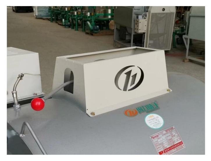
Top cooling switch design, after tea roasting processing, open the cooling valve, can accelerate heat dissipation.
