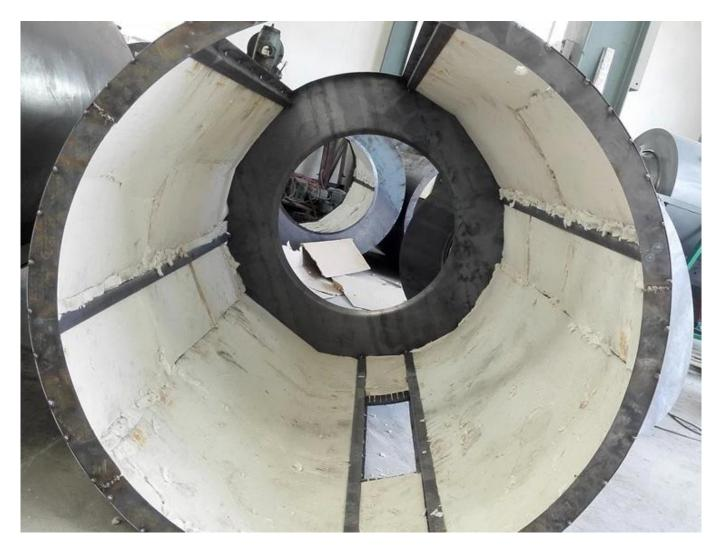
The inner barrel uses a new type of environmentally friendly fireproof insulation material, thickness up to 20mm, greatly reduces heat loss and saves energy by 30%.
