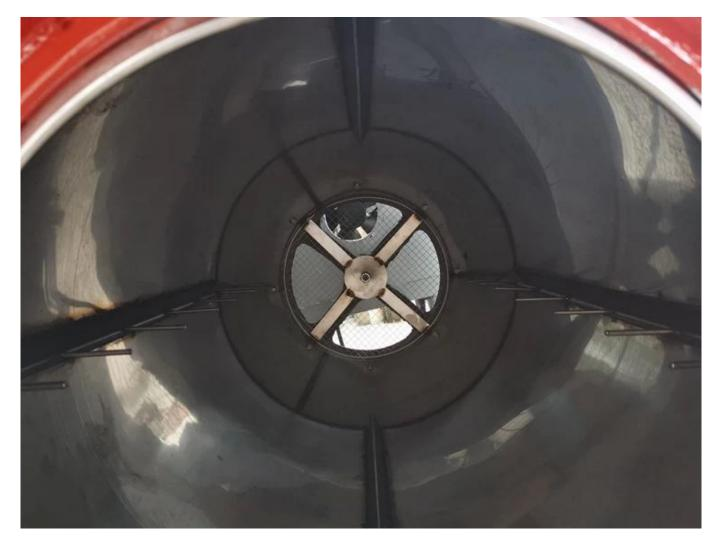
Using 2.5mm ultra-thick steel plate, the temperature change is small and good heat preservation, the tea leaf will not be damaged, ( other factory only use 1.6mm steel plate )
