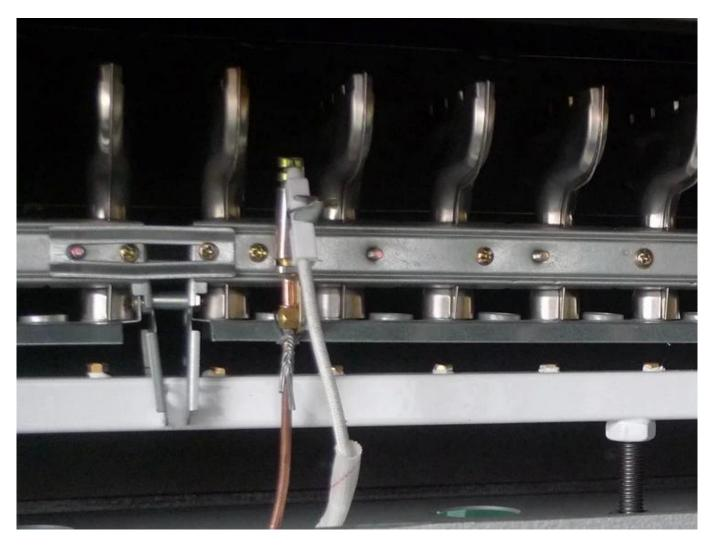
Preserve the design of the combustion head of the constant burning flame, reserve the constant burning flame after the ignition is successful, re-ignite from the constant burning flame, reduce the pressure of the ignition needle and the ignition coil, and improve the service life.
