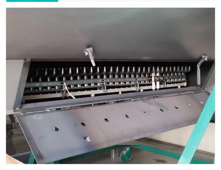
T-shaped combustion fire platoon covering the tea fixation barrel, burning area up to 100%.
