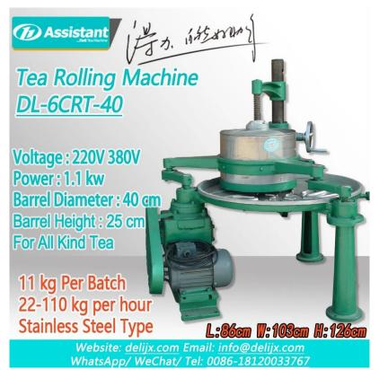
40cm Battel Middle Type Tea Twister Twisting Machine DL-6CRT-40
