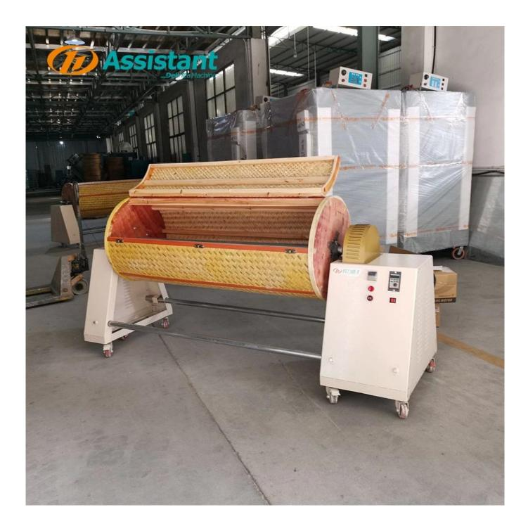
The bamboo door with holes can screen out the broken tea leaf dust during oolong tea tossing step, and can improve the quality of tea.
