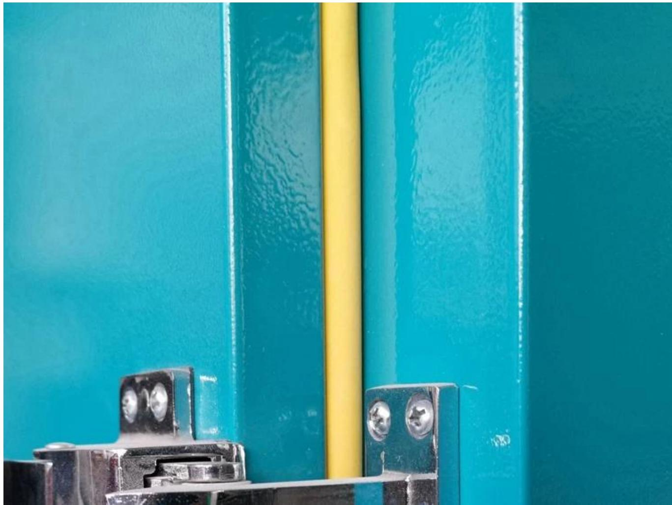
The door is lined with high-temperature resistant elastic rubber strips, which can seal the door of the machine to prevent hot air and water mist from escaping.
