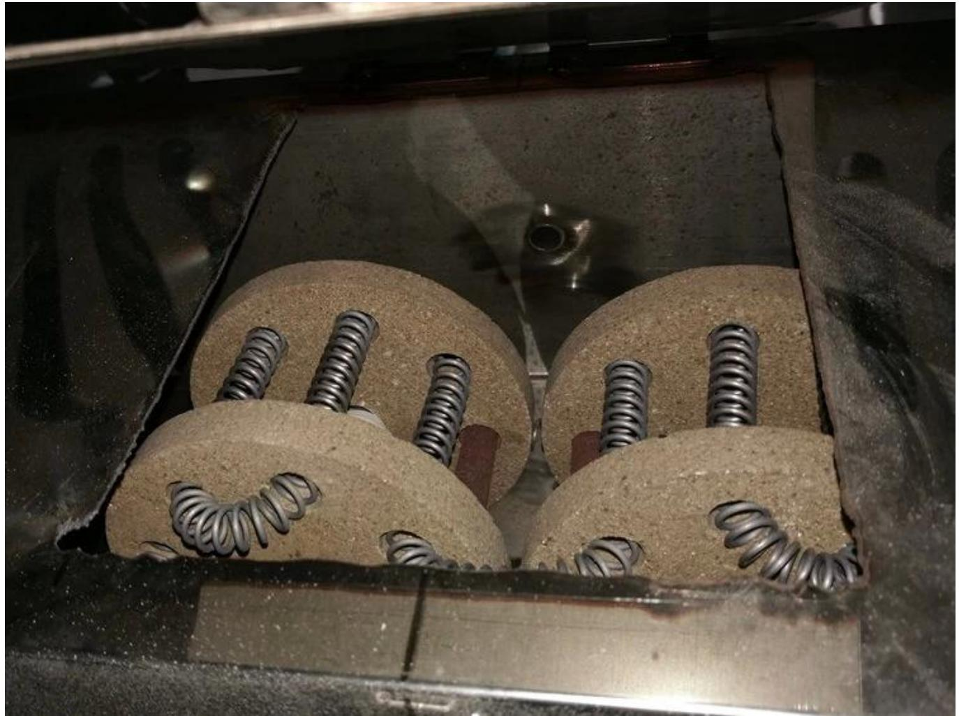
Using a durable electric heating wire with a diameter of 1mm and a high-temperature resistant polymer insulation cake, the service life of the heating wire is increased by 40% compared with other companies.
