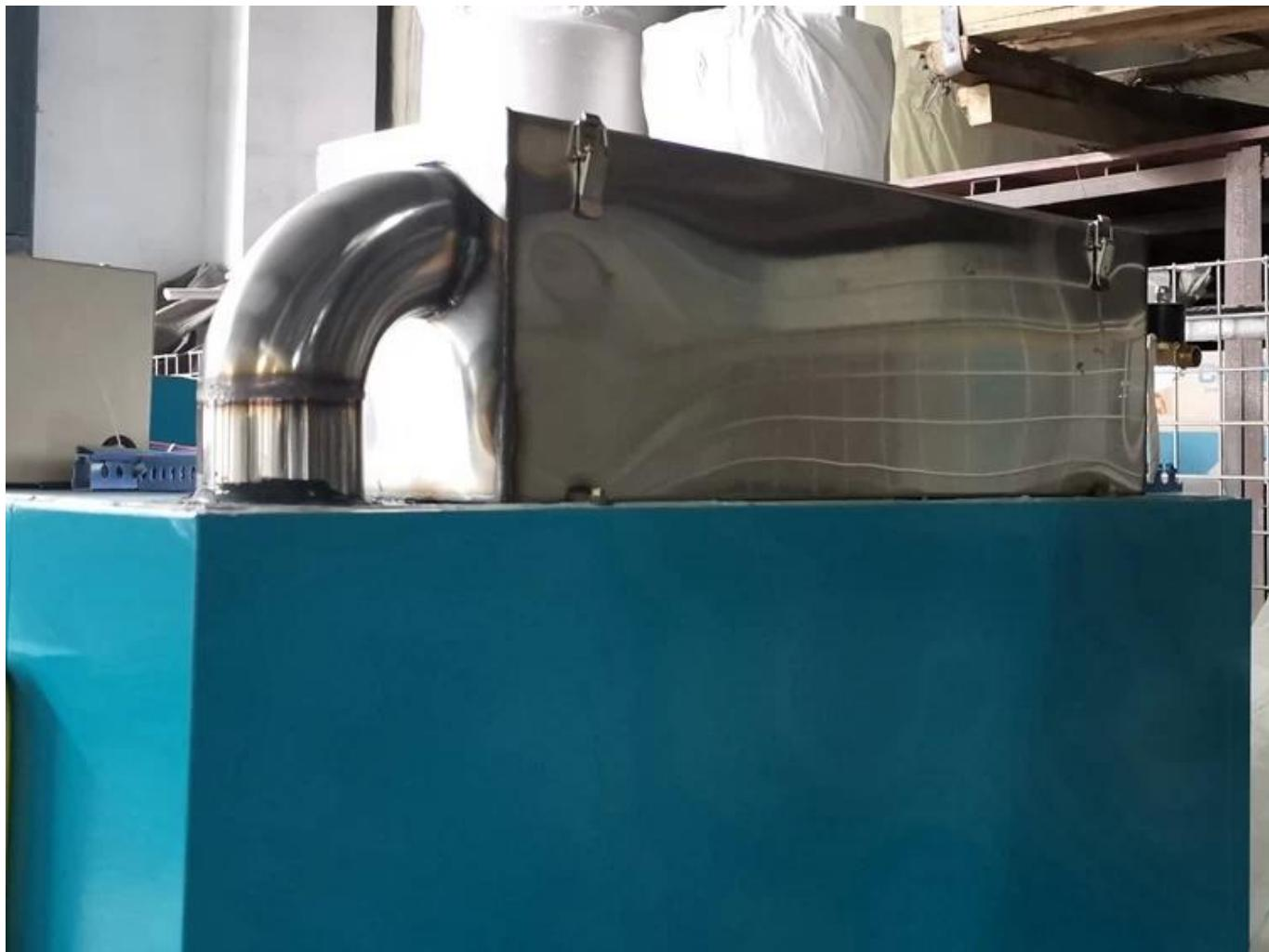
The water tank with atomizer is installed on the top, and the atomized water mist naturally fills the inside of the tea fermentation machine, and the fermentation is more uniform.
