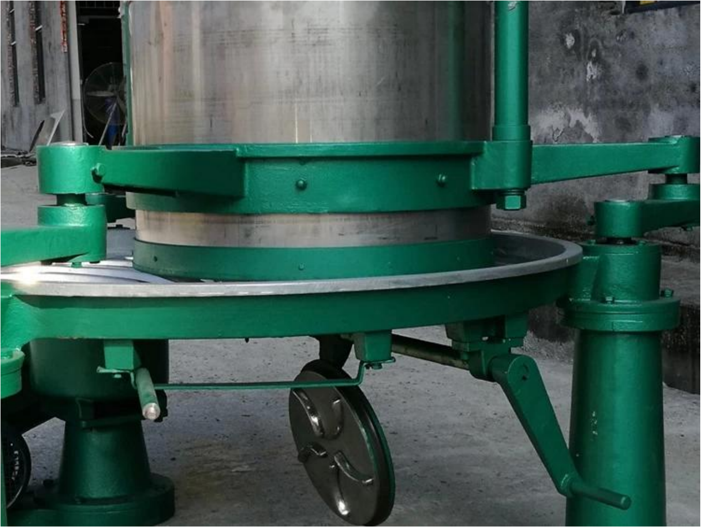
The supporting part of the machine is made of cast iron, which is strong and durable.
