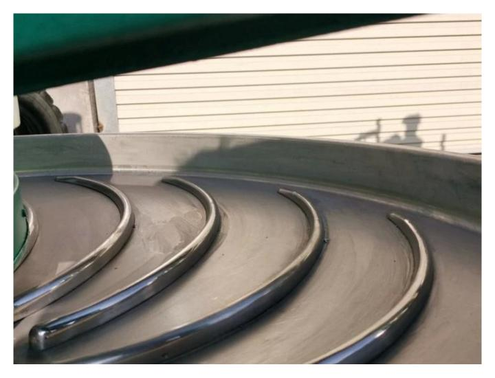
The heightened design of the rolling barrel can prevent the tea leaves from falling.
