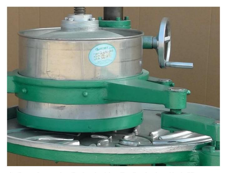
The distance between the rolling barrel and the rolling disc of each machine is different to ensure that each machine can make the best quality tea.
