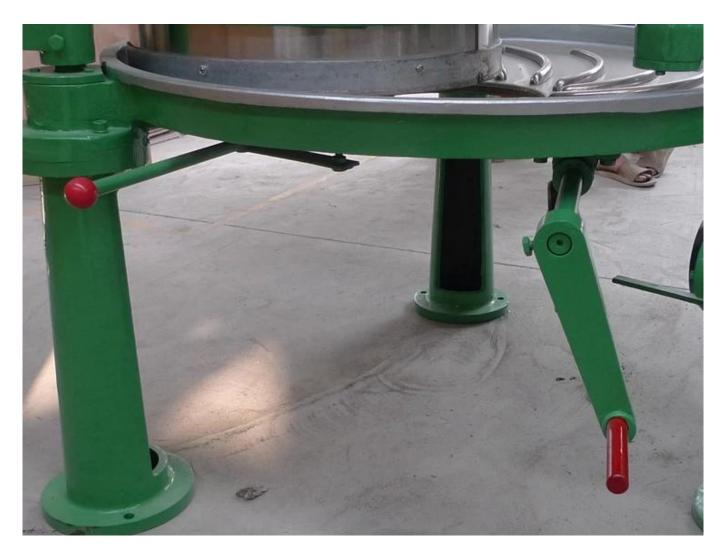
The bottom discharge handle design, gently push the handle, the tea can fall easily.
