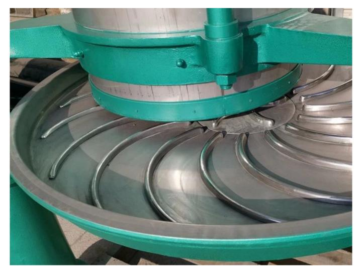
The arc of the rolling bar has been improved for decades, and the optimal design has been obtained. The efficiency of tea leaves been the strip-type is increased by 30%.
