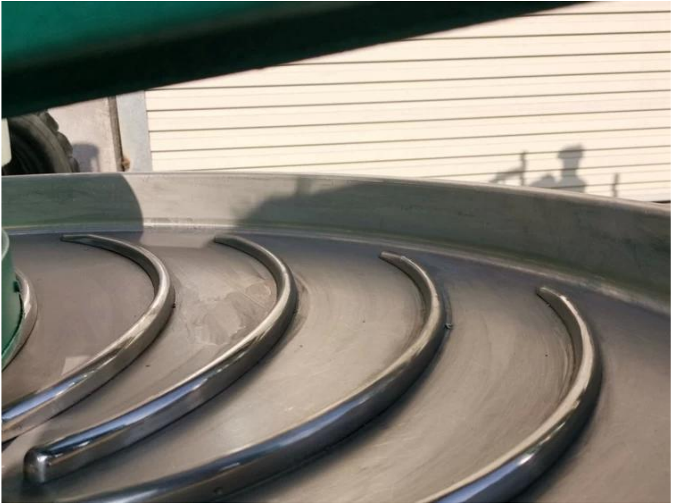
The heightened design of the rolling barrel can prevent the tea leaves from falling.
