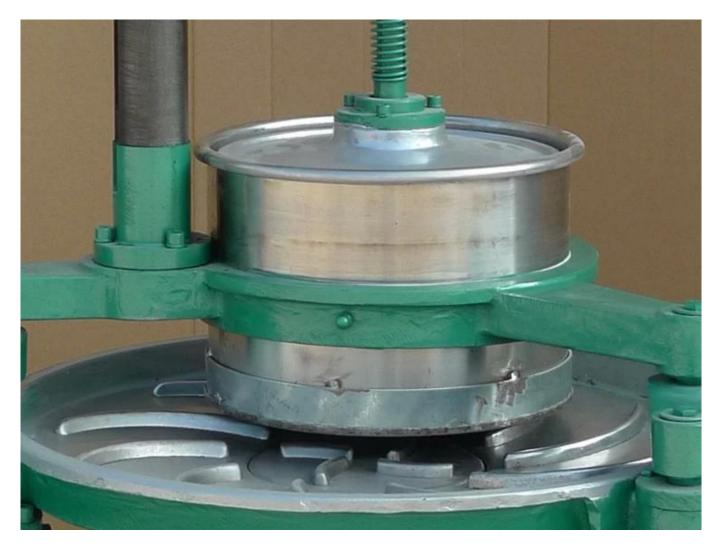
DL-6CRT-25 tea rolling machine drum diameter is 25cm, height 18cm, can put about 3kg per batch, for green tea processing, capacity is 3-30kg per hour, for black tea processing, capacity is 3-6 kg per hour.
