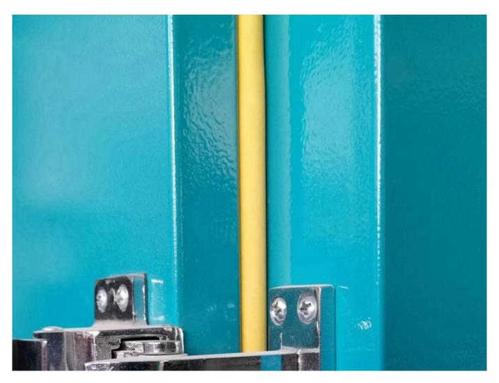
The door is lined with high-temperature resistant elastic rubber strips, which can seal the door of the machine to prevent hot air and water mist from escaping.
