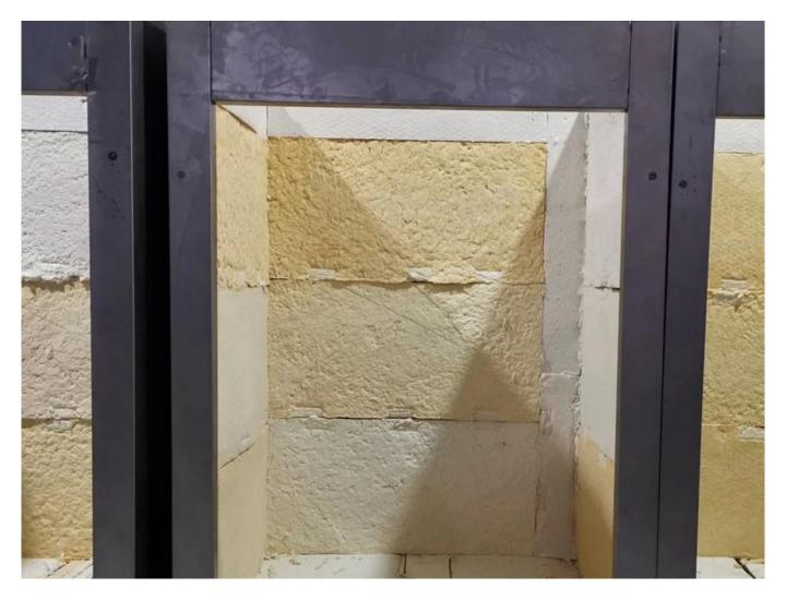
A new type of environmentally friendly high-temperature heat-resistant insulation material, with a thickness of 3 cm, and completely covering the machine to ensure that no heat is wasted and 30% energy saving.
