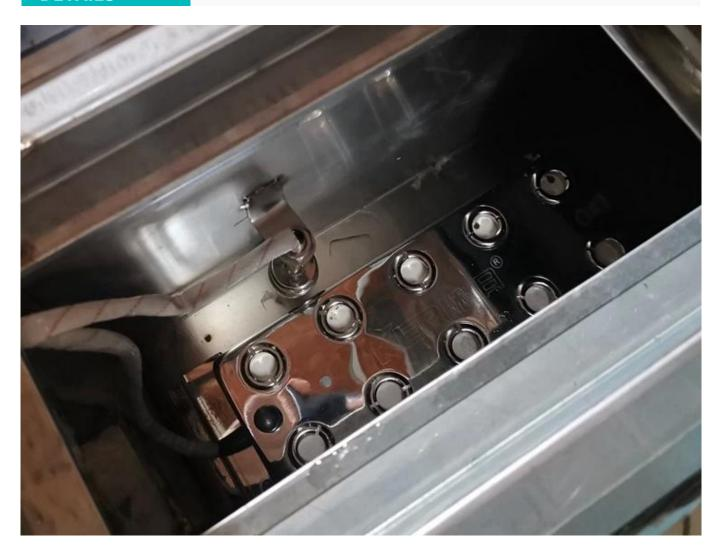
The high-frequency ultrasonic atomizer can atomize the water into very small droplets, which can enter the tea and improve the uniformity of fermentation.
