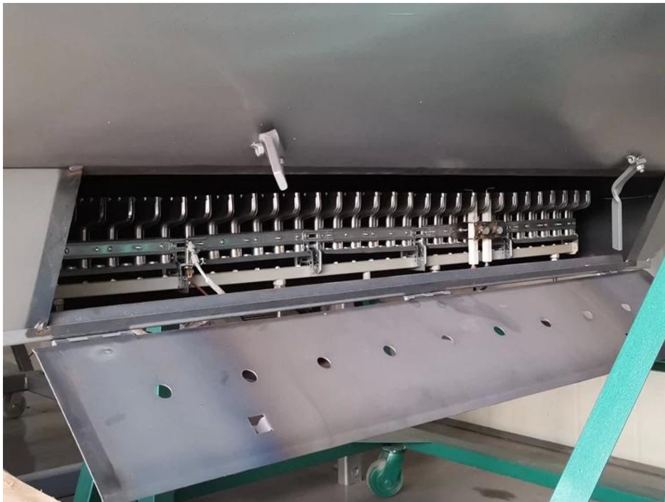
T-shaped combustion fire platoon covering the tea fixation barrel, burning area up to 100%.
