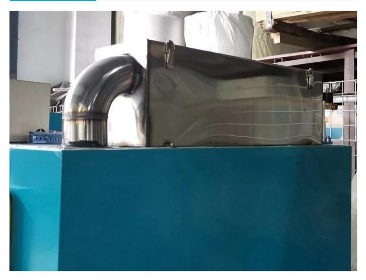
The water tank with atomizer is installed on the top, and the atomized water mist naturally fills the inside of the tea fermentation machine, and the fermentation is more uniform.
