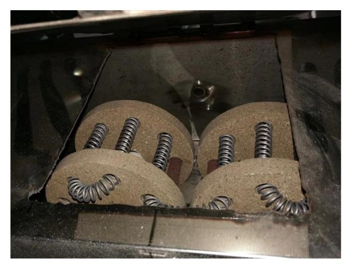
Using a durable electric heating wire with a diameter of 1mm and a high-temperature resistant polymer insulation cake, the service life of the heating wire is increased by 40% compared with other companies.
