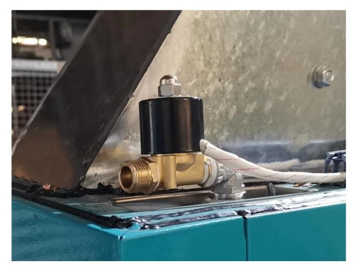
The solenoid valve design ensures that the water in the tank is kept at the best atomization height.
